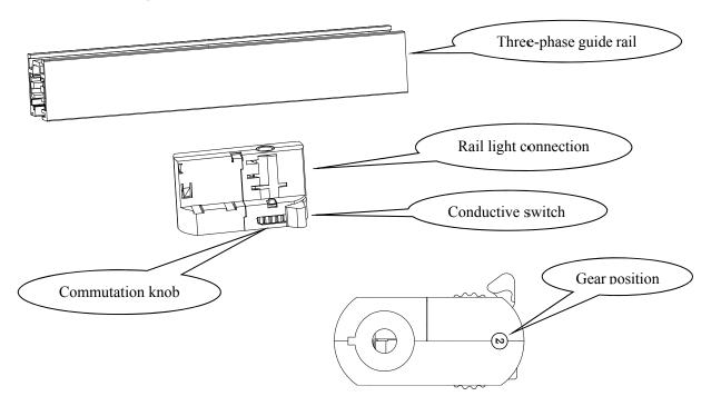
2. Align the protrusion of the rail light connector with the groove of the rail before assembly.
