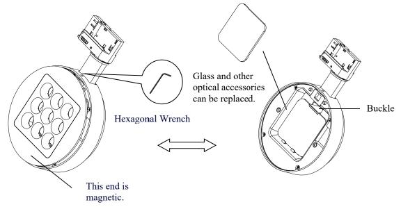
3. The installation sequence is the reverse of the removal sequence. Install the cover in the direction of the corresponding buckle, and it is considered to be installed when you hear a "click" sound and the cover of the lamp has no protrusions.
