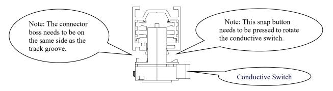
3. After assembly, turn the "Conductive Switch" clockwise by 90 degrees to conduct.
