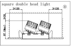
2. Cutoff  $\phi$  75mm circular hole on the ceiling, see4; Cutoff 75\*75mm square hole on the ceiling for square light, see5; Cutoff 146\*74mm square hole on the ceiling for square double head light, see6.
