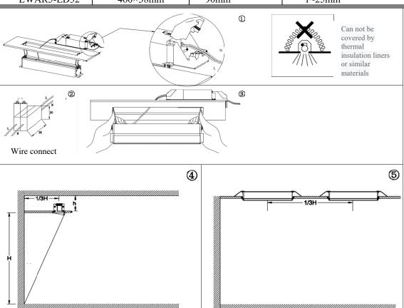
\* If the driver of the light comes with lead wires, and the leads need to be connected with an independent terminal block (refer to Figure 3 for wiring), the size of the terminal block for each line should not be less than 10x20x25mm.
