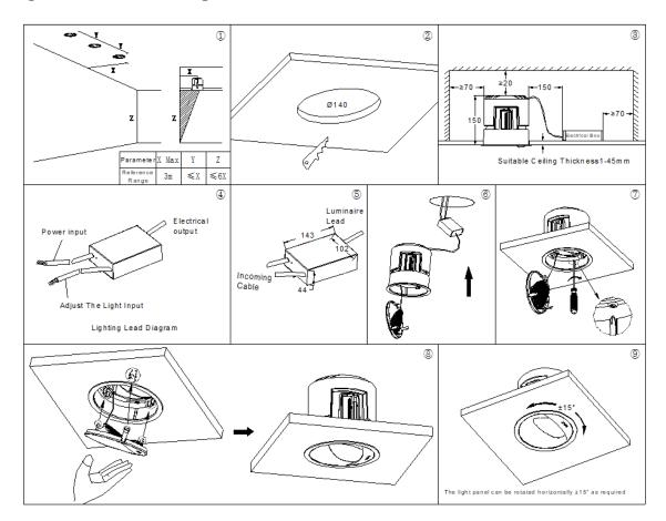
\* Note: Connect the cable according to the voltage requirements of the power line input label; If there is a dimmer version, please pay attention to the light +/- pole, do not connect the wrong. Pay attention to waterproof treatment of cable joints.
