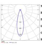
MODEL: DLT31-LM13E-230SWT BEAM ANGLE: POWER: 15W LUMENS: 896lm CBCP: 3065cd EFFICACY: 60lm/W
