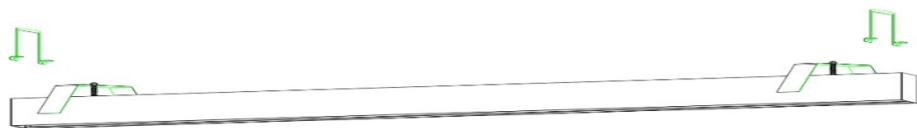
b. When loading the ceiling, first load one end of the lamp body into the ceiling, and then install the other end, pay attention to the ceiling hole ruler
