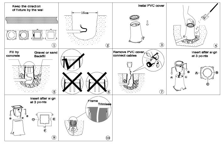
2. Recessed (Not suitable for the trimless fixture)
