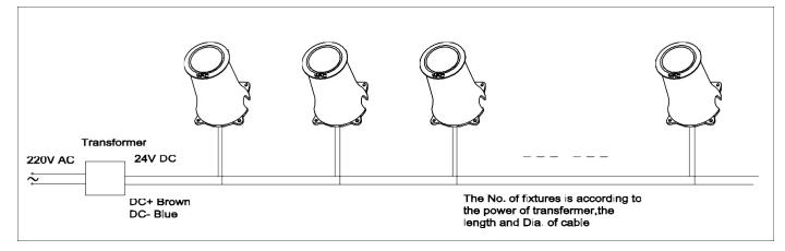
5. The relation of the fixtures' QTY., the transformer 's power, the length and Dia. of cable show as below:
