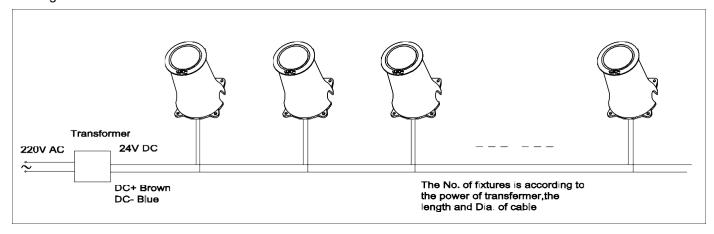
5. The relation of the fixtures' QTY. ,the transformer 's power, the length and Dia. of cable show as below:
