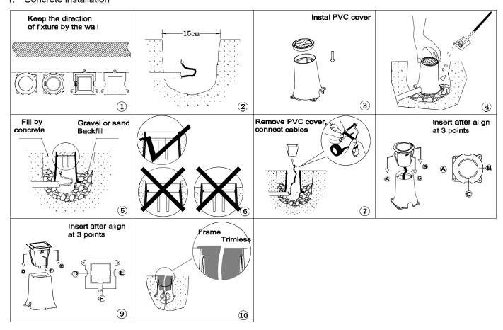
2. Recessed (Not suitable for the trimless fixture)
