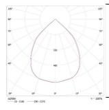
Model: EP6SI-070EL-830BK Beam Angle:82.8° System Power:70W(Max) System luminous flux:7669 lm Central light strength:/
