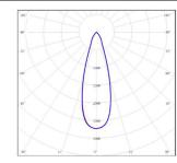
Model: EP4LI-54EL-330BK Beam Angle:33° System Power:54.6W System luminous flux:5708 lm Central light strength:/ System light efficiency:104.5 lm/W
