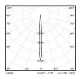
Model: EP4NI-10EL-130BK Beam Angle:15° Light source Power:10W System luminous flux:850 lm
