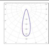
Model: EP4MI-30EL-230BK Beam Angle:27° System Power:30W System luminous flux:2647 lm Central light strength:/ System light efficiency:88.3 lm/W
