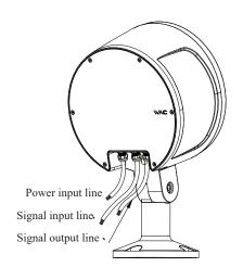
DMX512Signal line label Yellow green line: Gndground wi Red line: DMXSignal input positive black line: DMXSignal input negative 4. The power input is AC220V, and the product is DMX512 dimming lamp wiring method:
