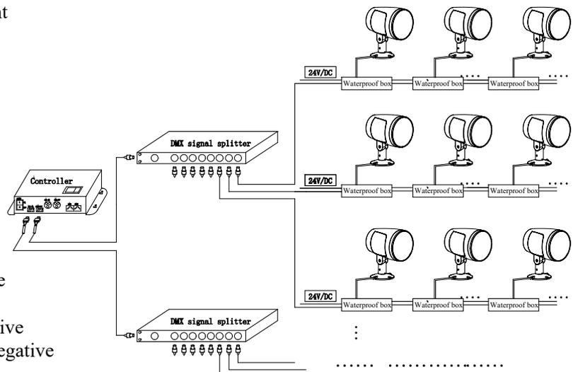
4. Connect all lighting fixtures to a control network and adjust control as needed
